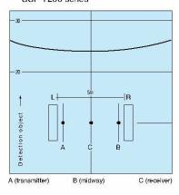
Smallest detectable object diameter characteristics SSF-T400 series
