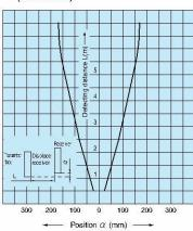
Parallel displacement characteristics (Horizontal) (All models)
